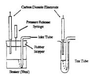
1. Bubble the 5% gas through the chamber and record the millivolt value after a stable reading is obtained. It may take up to 15 minutes to de-gas the chamber of contaminants. However, bubbling the gas vigorously will cause droplets to collect on the tip of
