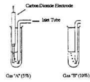
Calibrating standards and samples must be at the same temperature for accurate Carbon Dioxide measurements.
